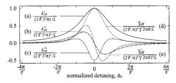
FIG. 3. Functional dependence of (a) the group velocity reduction, (b) group velocity dispersion, (c) third-order dispersion, (d) Kerr coefficient, and (e) self-steepening coefficient on the detuning for a SCISSOR. The parameters have been scaled such that the curves are universal and fit within the same plot limits.
