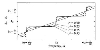
FIG. 2. Dispersion relation for light propagation in a SCISSOR with differing values of the self-coupling coefficient r.  $k_{\text{eff}}-k_0$  is the resonator contribution to the propagation constant.
