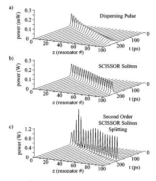
FIG. 4. (a) A weak pulse propagating in a SCISSOR disperses. (b) A pulse with amplitude corresponding to the fundamental soliton propagates without dispersing. (c) A higher-order breathing soliton is unstable under the influence the resonator-induced intensity-dependent group velocity (self-steepening).
